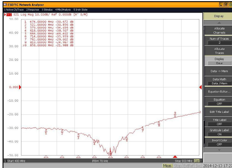
Isolation RF FWD vs RF RFL
